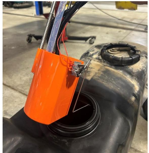
**Model Years 1999-2003 7.3L Powerstroke:** Orient the SureFlo sending unit to where the indented mark on the cap lines up with the notch in the tank flange as shown at right.
