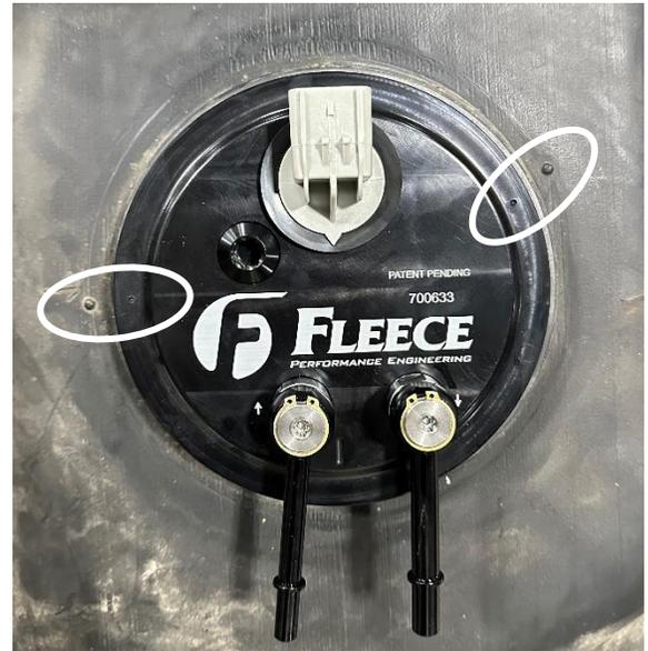
**STEP 13:** Place the tank back on the jack and lift the tank until it reaches around five to six inches short of its installed position. Reconnect the fuel lines. Connect the harness adapter to the SureFlo sending unit. Connect the OE electrical harness connector to the end of the adapter.
