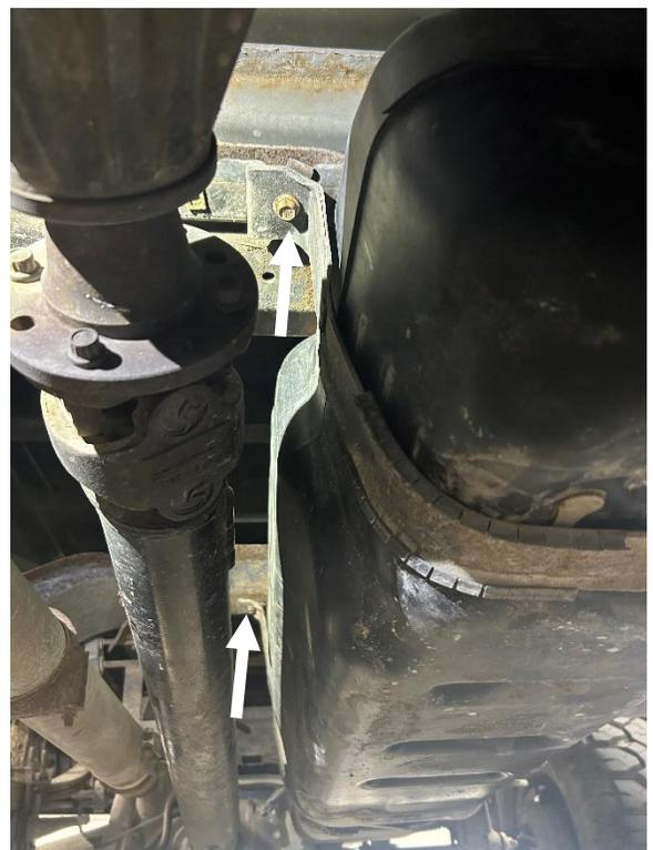
**STEP 6:** Lower the tank five to six inches and disconnect the electrical harness connector for the sending unit. Using a 3/8" quick disconnect tool, remove the fuel feed connector (blue quick connect fitting shown at right). Using a 5/16" quick disconnect tool, remove the fuel return connector (white quick connect fitting shown at right).
