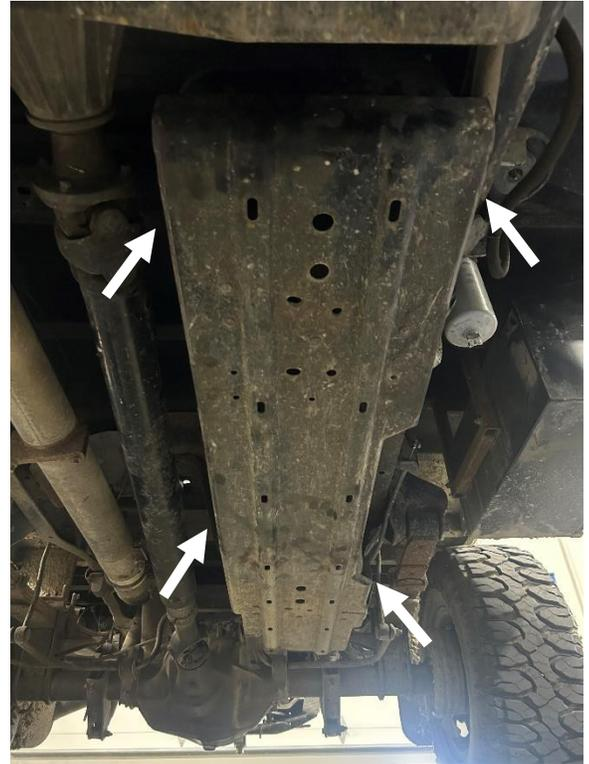
**STEP 5:** Place a transmission jack or floor jack under the fuel tank to lightly support it. Remove the two bolts retaining the tank straps using a 13mm socket or wrench.
